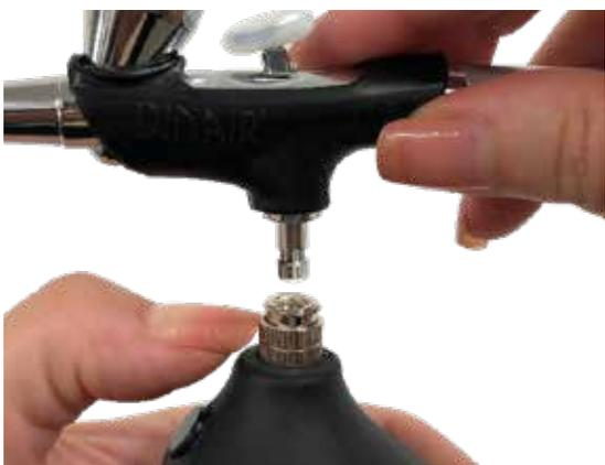
Push spring clasp collar down to release airbrush.
