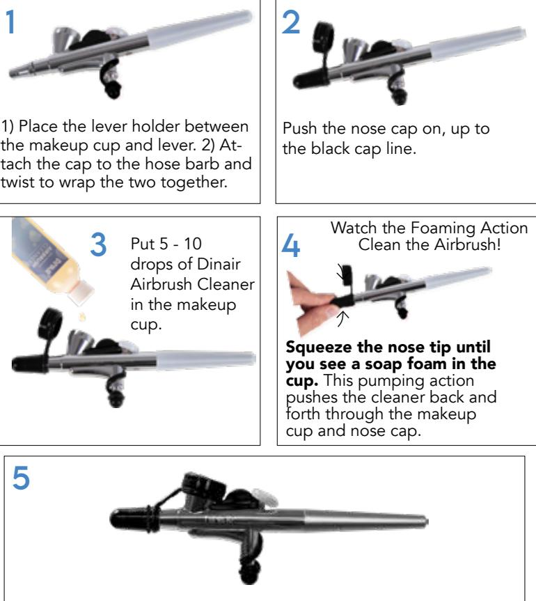
**1** Place the lever holder between the makeup cup and lever. **2** Attach the cap to the hose barb and twist to wrap the two together.
