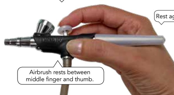
Hold the airbrush as you would hold a pen, with gentle grip and fingers extended. Find a comfortable grip and place your index finger on the lever. Use your index finger to pull back on the lever gently. Never use your thumb to control the lever.
